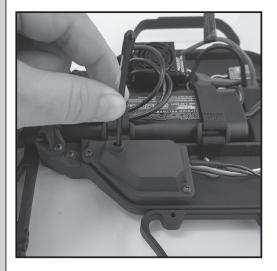
Install antenna wire through antenna tube, then install antenna tube as shown.
