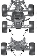
\*Front arms inner and outer hinge pins should be in a imaginary horizontal line when ride height is set
